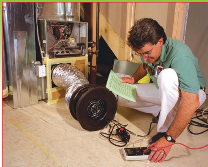
In this photo, a Building America staff member performs a duct blaster test to measure the impact of duct leakage on whole-house performance.
