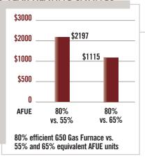
This chart depicts potential energy savings you can expect from the G50 gas furnace versus older furnaces with lower efficiency ratings. Criteria used in this example are 2,000 full-load heating hours, with a 60,000 Btuh heating design load and \$1.074 ccf for gas. Your actual savings may vary depending on the weather, local fuel rates and your lifestyle. AFUE = Annual Fuel Utilization Efficiency.
